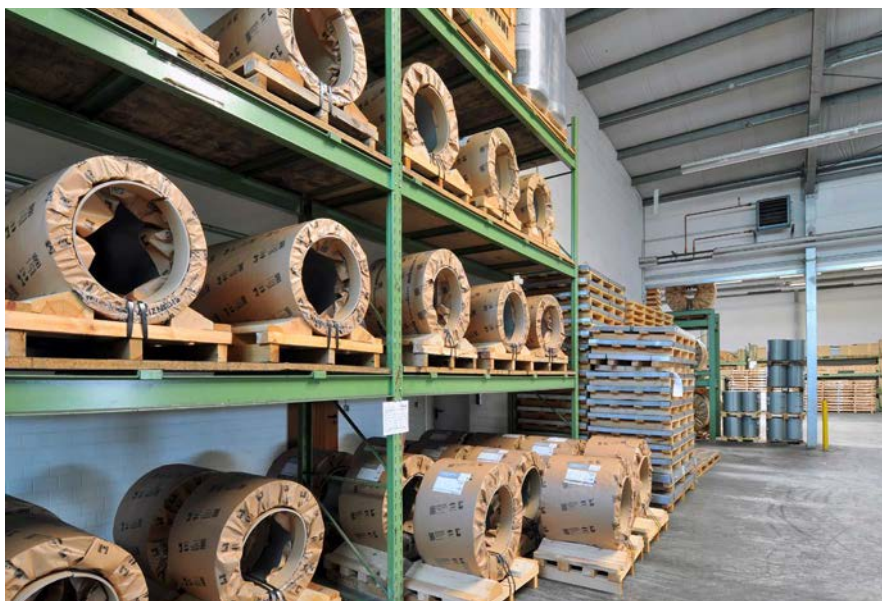
Storage of coils with wooden sleepers
